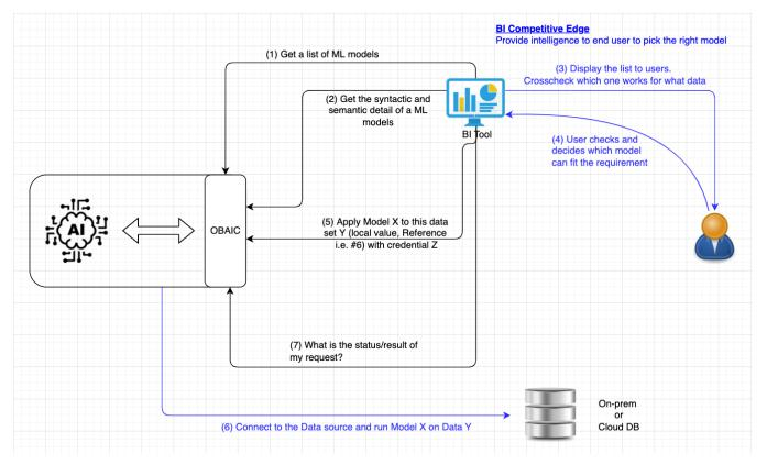
1. When a BI user wants to extend its capability to AI, it reaches out to AI platform and requests a list of available models of which the credential of the provided token is authorized to see
