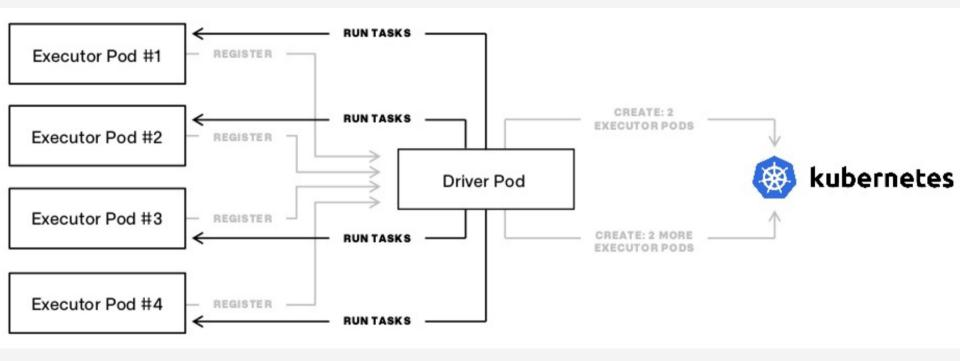
The SparkJob operator supports parallel processing on multiple nodes
